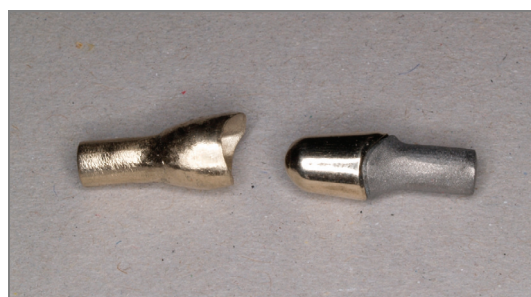
Fig. 1b. Sample of primary and secondary cast crowns prepared for testing
