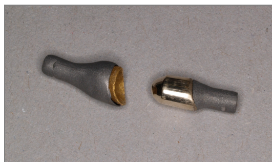
Fig. 1a. Sample of primary cast crown and secondary electroformed coping prepared for testing
